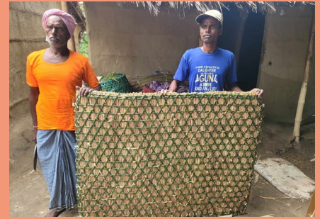
There, residents and artisans worked together to test different thatch panel options for ceilings.
