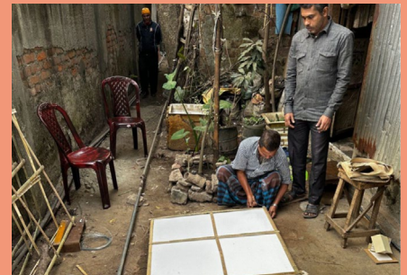
In Dhaka, inexpensive insulation panels were tested as removable layers to reduce heat gain.
