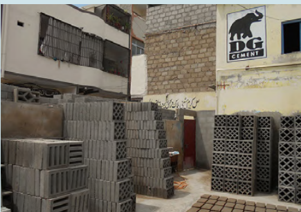
Concrete lattice elements commonly used in Karachi.
