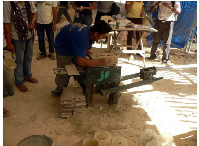
The three block-making machines at LTHAI could produce 1,050 blocks per day, with three teams alternating in two shifts.
