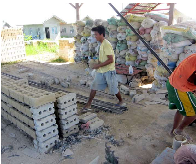
These are some photos taken in April 2004, when the interlocking concrete earth blocks (ICEBs) were being manufactured on the site, in preparation for building the new houses.
